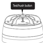
**NOTE:** The reason of this is that it is necessary to locate the source of the alarm before using the hush function. This is to make sure that it is not a life threatening situation.
